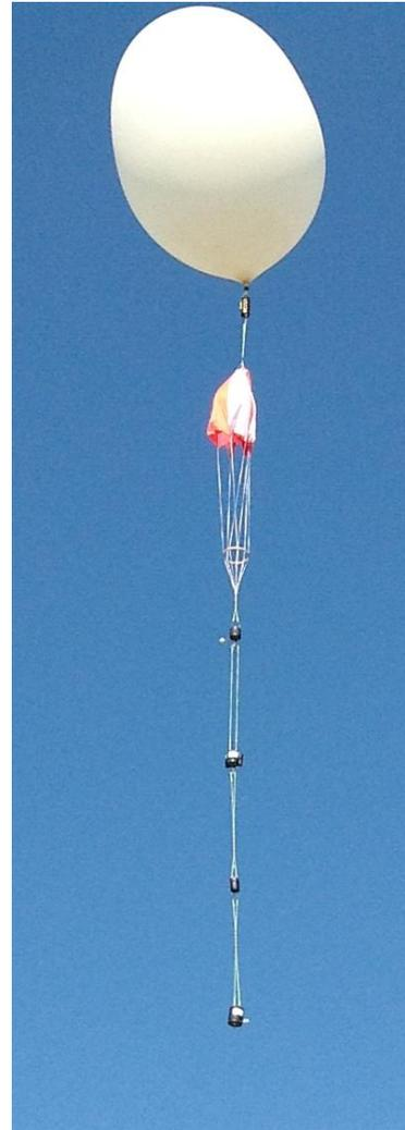
**Fig. 3-4 Flight 282 at beginning of launch showing four PODS and the parachute with an enclosed 100g balloon. The internal probe boom is not visible but is located inside the balloon.**
