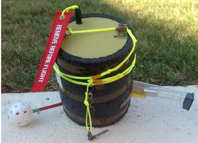
**Fig. 3-3 Temperature POD with calibrated MET unit (with plastic protective cover) and diode temperature sensor in white plastic hollow ball with holes for convection.**
