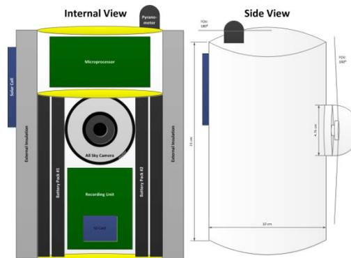
**Figure 3.** Mechanical Diagram. Pod structure of Flight #2 with sensors from Flight #1
