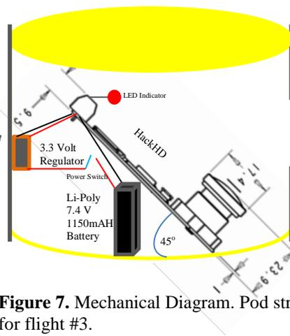
**Figure 7.** Mechanical Diagram. Pod structure for flight #3.
