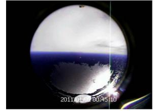
**Figure 12.** Shot in mid-flight with frost on encasement and wrong orientation.
