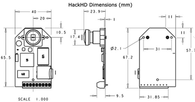
**Figure 6.** The dimensions of the HackHD in mm
