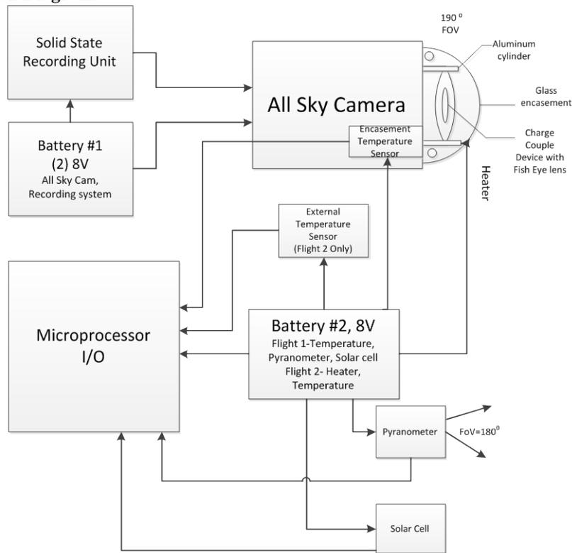
**Figure 1.** Block Diagram of both Flight #1 and Flight #2 (System varies per flight)
