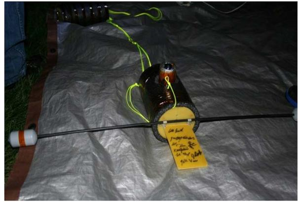
**Figure 5.** The finished pod with the inertial booms and tail about to launch. We also signed the tail for that personal touch for Flight #2.
