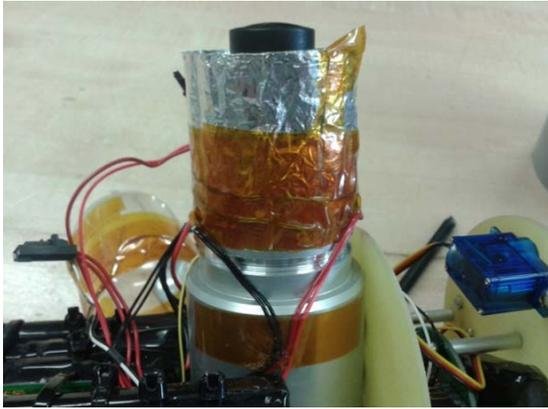
**Figure 4.** The Niacrom wire wrapped around the aluminum and connected to the batteries for Flight #2.
